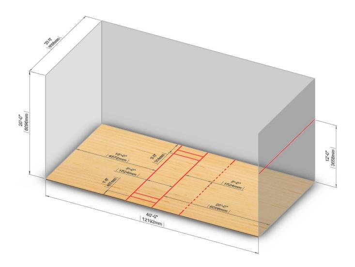
**1.2 General Configuration of a Convertible Court.** The general configuration of a convertible court shall be as shown below (see detail for floor markings):
